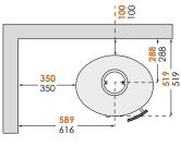
In order to avoid discolouration of painted and treated surfaces, TermaTech recommends the same distance from flammable materials as for non-flammable materials. This distance increases the convection itself around the stove and also eases cleaning. All distances relate solely to the distance of the stove from flammable materials. No account has been taken of national requirements for the use of stove flues or their distance from flammable materials.
